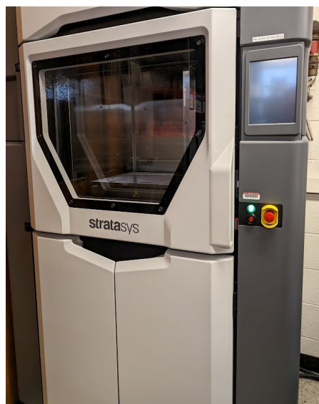
Large Format FDM Printer
