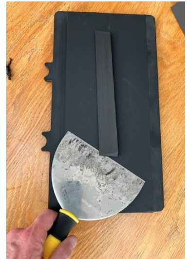
Image 1: Person loosening the print from building plate with a scraper.
