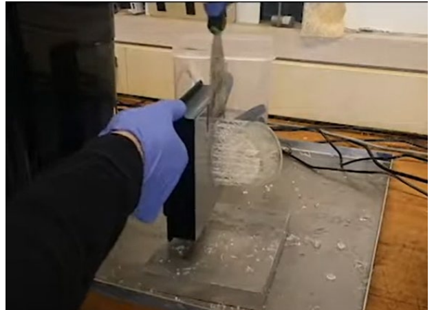
Image 2: Build plate affixed to fixture to safely remove print from build plate.
