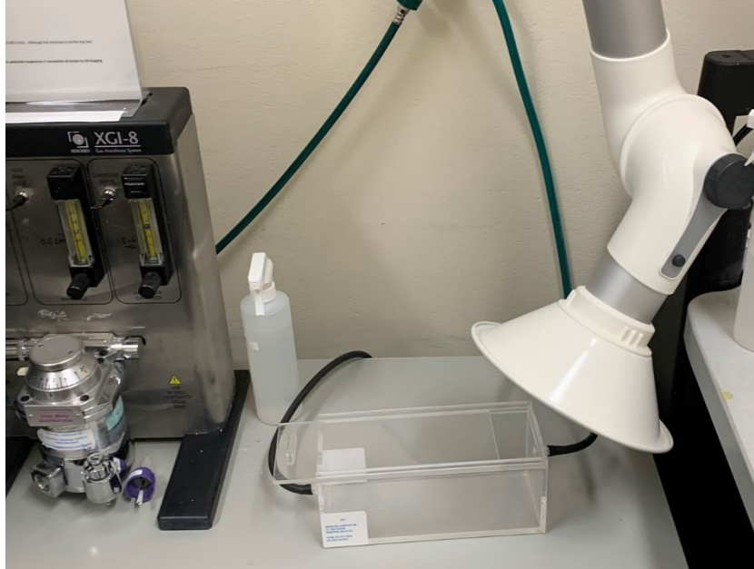
Image 20: Exhaust snorkel close to the induction chamber for better isoflurane capturing
