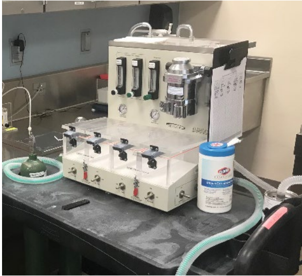
Image 7: Induction chamber with passive scavenging Canisters
