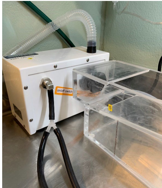
Image 19: Pumped induction chamber with sliding door
