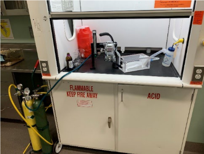
Image 15: Isoflurane induction chamber inside a fume hood
