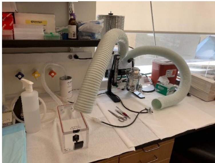
Image 14: Benchtop gas/vapor snorkel connected to the carbon filter/HEPA
