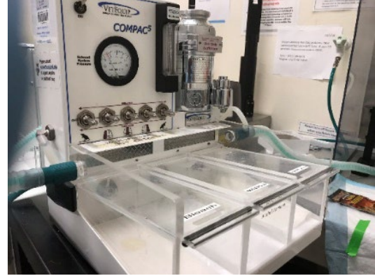
Image 4: Induction chamber chambers connected to active scavenging system
