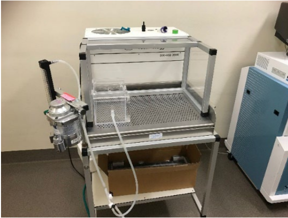
Image 12: Downdraft enclosure with carbon filter chamber
