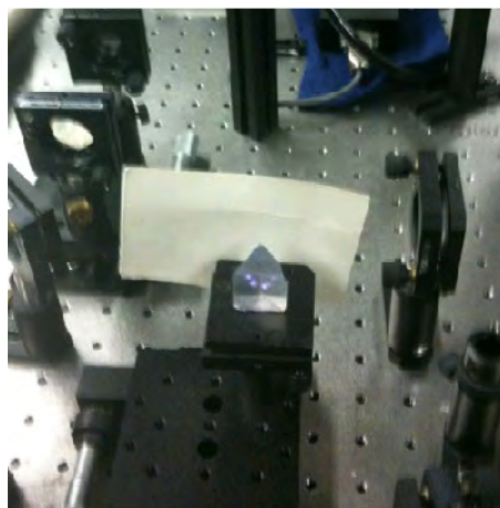
Figures: Ad hoc beam block made from a piece of paper (left) and duct tape (right)
